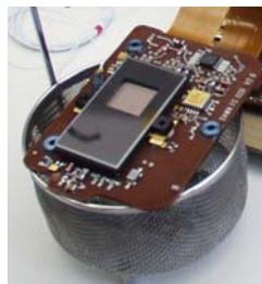
The selected sensor is a Thomson TH 7888A, a 1024 x 1024 pixel frame-transfer CCD. This is a commercial device equipped with an electronic shutter. Its high performance enables a 1.3 ms frame transfer, minimizing the frame transfer smear.
