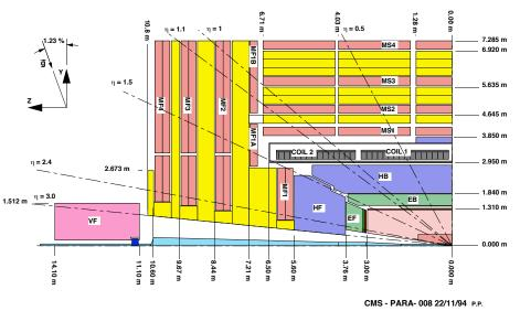
Largely extend the acceptance (rapidity from  $\sim 2.5$  to  $\sim 4.0$ )  $\rightarrow$ lower x in parton kinematics!
