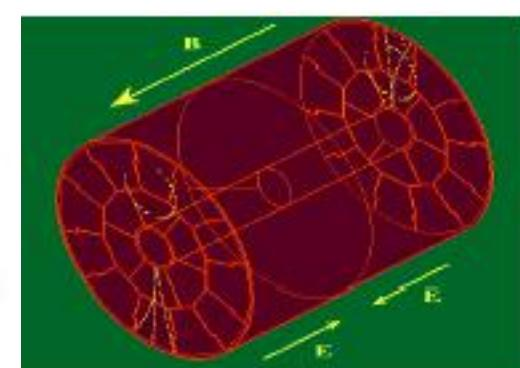
→ GEM+Micromegas hybrid detector to significantly reduce TPC ion back flow
