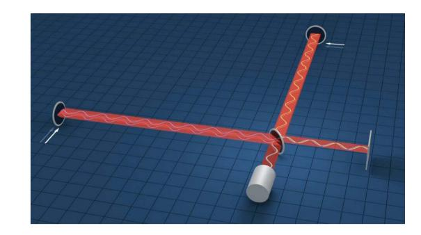
In a Michelson interferometer, variations of the light time travel in the perpendicular arms are converted into changes of the interference pattern at the output port of the instrument
