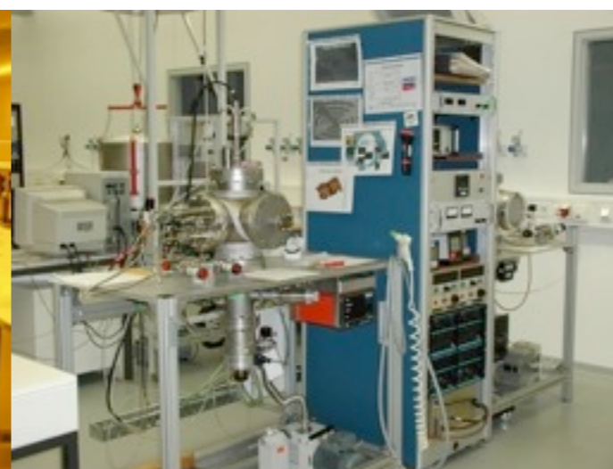
Production of thin NbN-films with reactive magnetron sputter (IMS)
