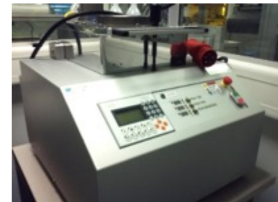
Vacuum reflow process with formic acid option
