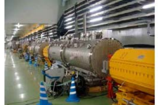
Installed Kicker Magnet
