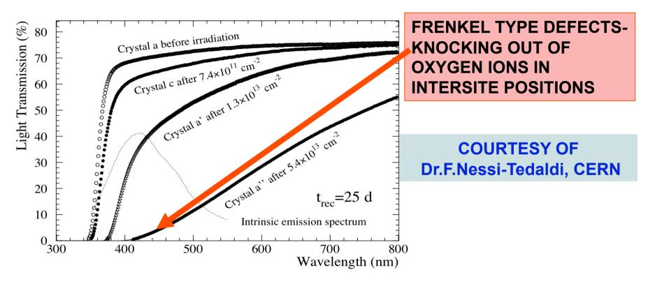
Optical transmission spectra of PWO crystal change after irradiation with protons .
