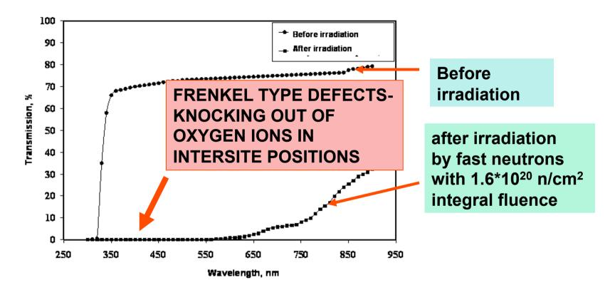
Optical transmission spectra of 0,2 mm PWO crystal after 1.6\*10<sup>20</sup> n/cm<sup>2</sup>
