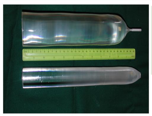
PWMO scintillator electromagnetic calorimetry
