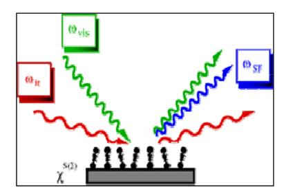
Chemical species can be identified and molecular surface density can be measured with this technique.
