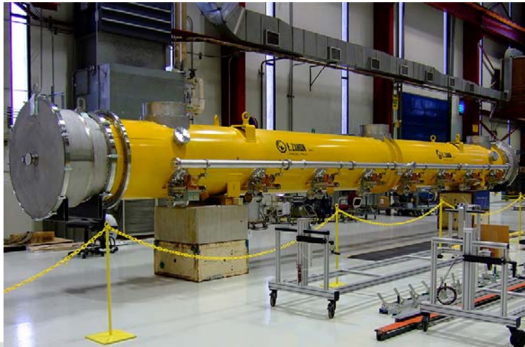
Cryomodule built at FNAL with DESY cooperation
