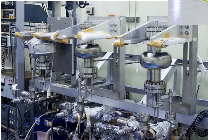
Single cavity tests at KEK
