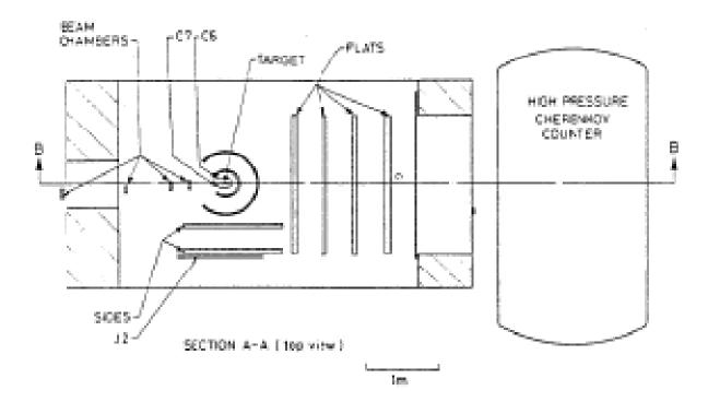
The Rutherford Multiparticle Spectrometer at Nimrod was equipped with chambers to measure tracks in magnetic field and a large Cherenkov counter for particle discrimination
