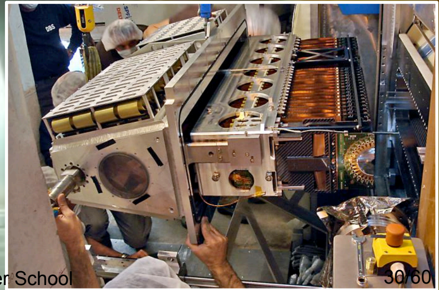
A VELO half during installation
