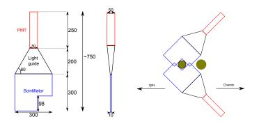
Size of scintillating plates choosen to be 300mm and the cut-out is the same as the trackers 98mm.
