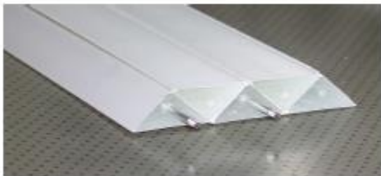
Triangular shaped bars (1.1m long, from Fermilab)
