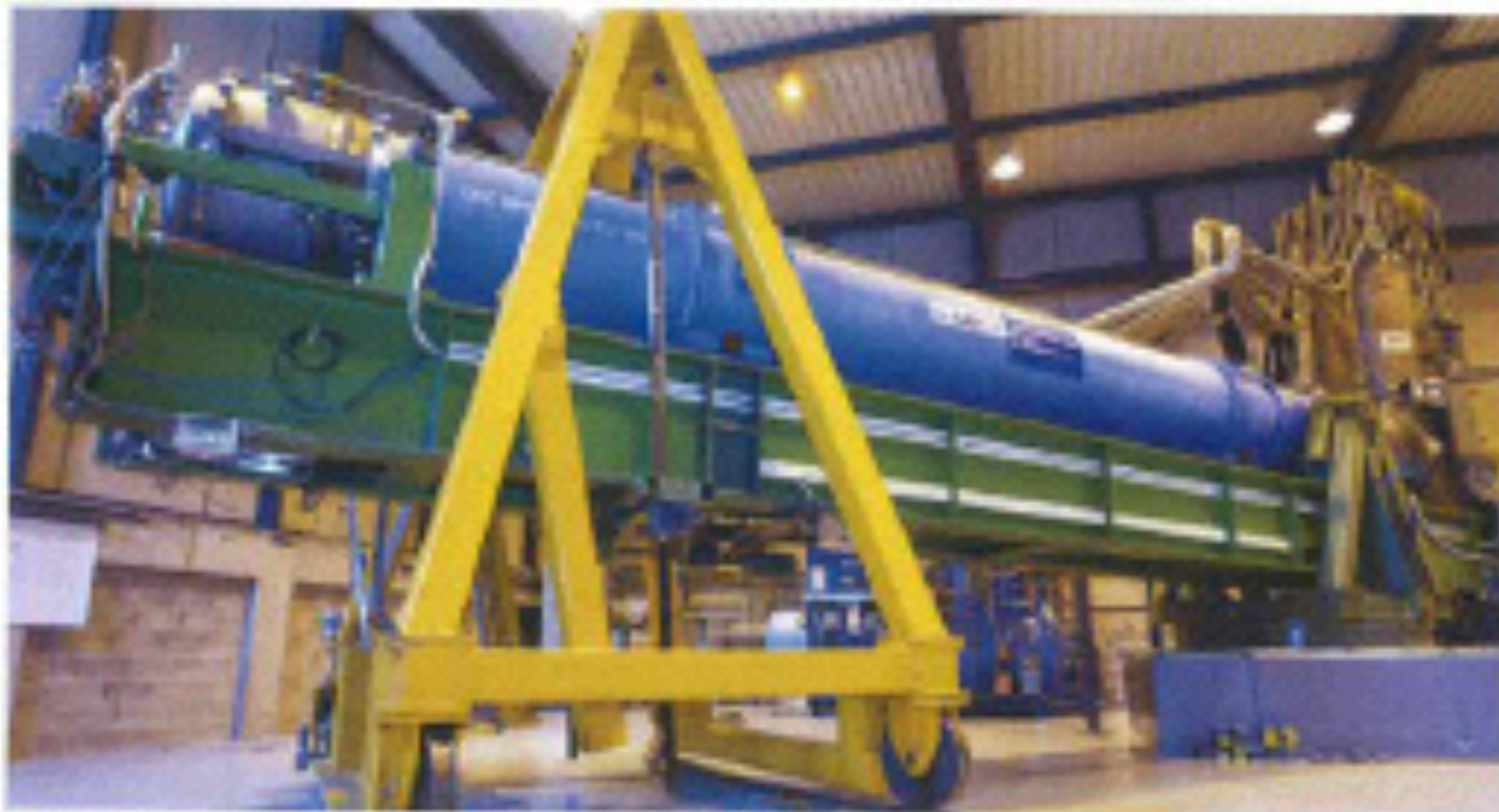
CAST, CERN's axion solar telescope, moves on its rail to follow the Sun (for an hour and a half at dawn and an hour and a half at dusk).
