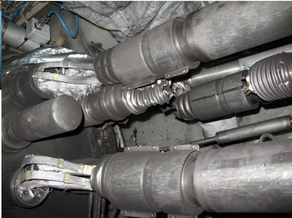
QBQI.27R3 Bellows torn open
