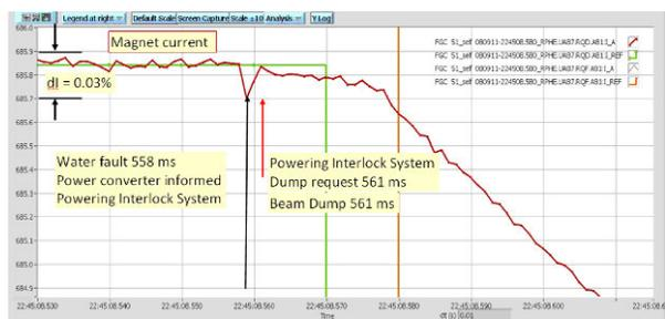
Figure 3: Event sequence of interlock signals, following a water fault in the DC cable of the defocusing quadrupole magnet chain of sector 81.
