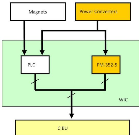
Figure 2: Functional architecture of the WIC interface with the Beam Interlock System, with the PLC and the Fast Boolean Processor 352-5 connected in parallel.
