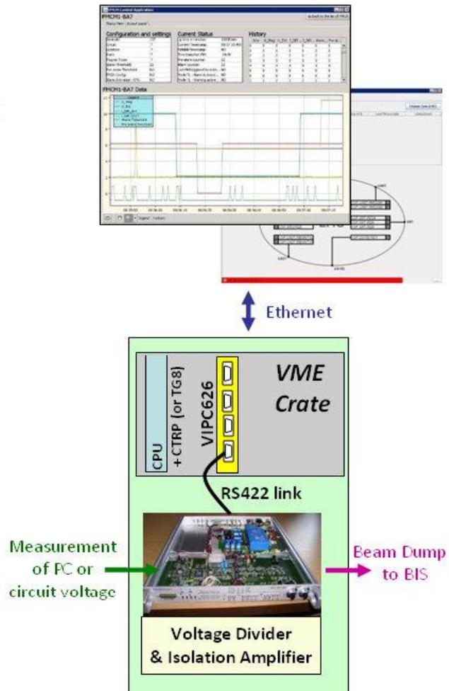
Figure 1: Vertical slice illustrating the integration of a FMCM into the CERN (controls) environment.
