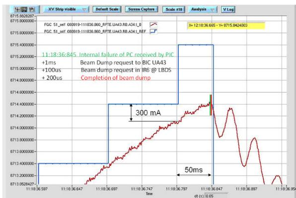
Figure 4: Event sequence of interlock signals, following the incident in the main dipole circuit of sector 34.
