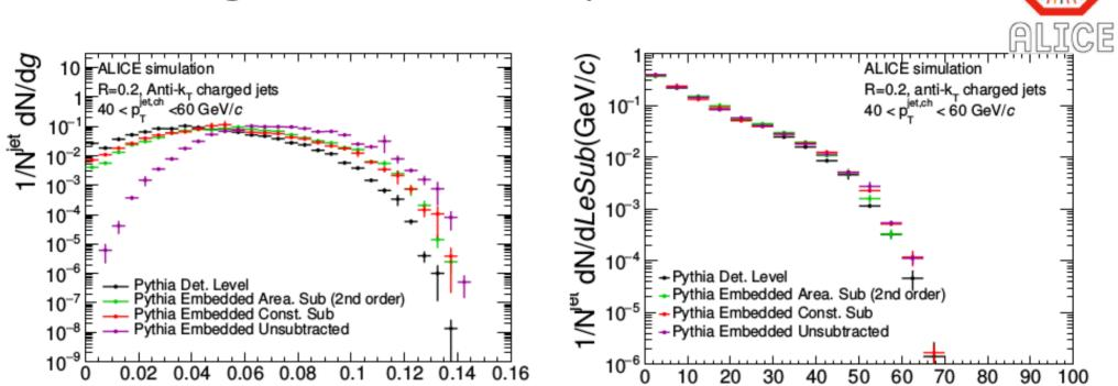
Pythia detector level jet embedded into Pb-Pb events and background subtracted
