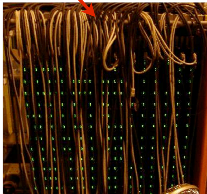
Analog HCAL 3 \times 3 - 12 \times 12 \text{ cm}^2 lateral segmentation 38 layers, \sim 4.5 \lambda \sim 8 \text{ k} channels
