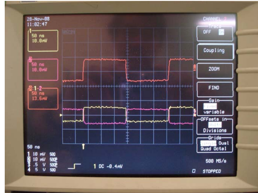
DeltaV, low gain, Cal- AFE bypass (the calibration signal don't goes inside the amplifier box)
