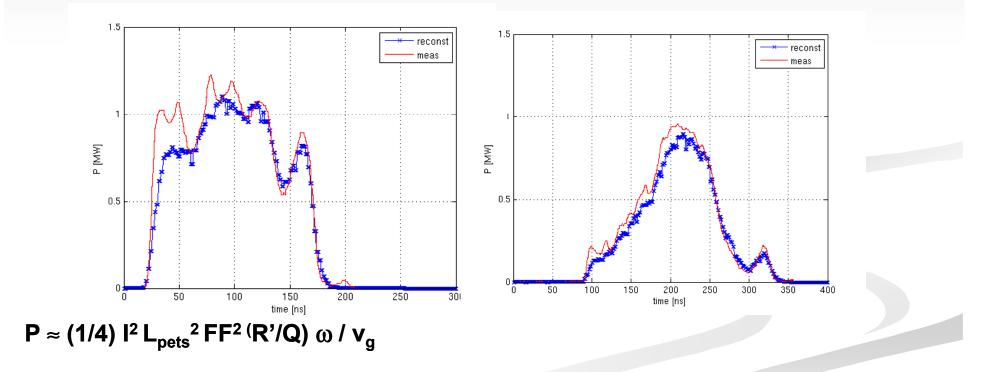
Apart from PETS parameters (tested with RF), the power should depend only on the form factor, the current<sup>2</sup> and eventual phase detuning.
