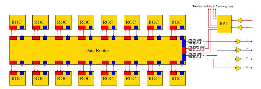
Phase I upgrade of the CMS pixel detector: FF-LYNX based TTC distribution and DAQ with trigger based individual ROC readout  $\rightarrow 4 \times 160$  Mbps optical fibers available for DAQ and reduced latency of data readout data (w.r.t. token based readout)
