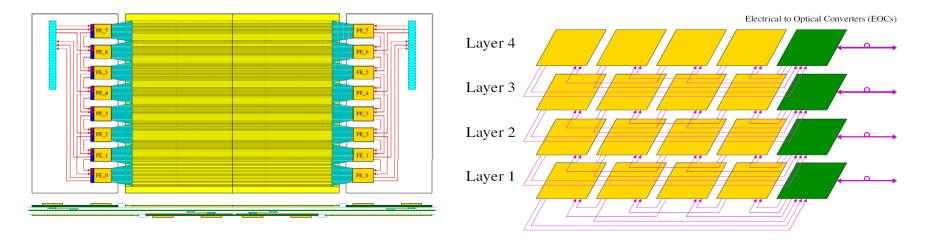
Phase II upgrade of the CMS Strip Tracker (no trigger data readout): daisy chains of Front-End ASICs within the modules and, optionally, daisy chain of modules. Expected data rate for raw data, at r = 78 cm: 5 Mbps/FE chip  $\rightarrow$  40 Mbps/module.
