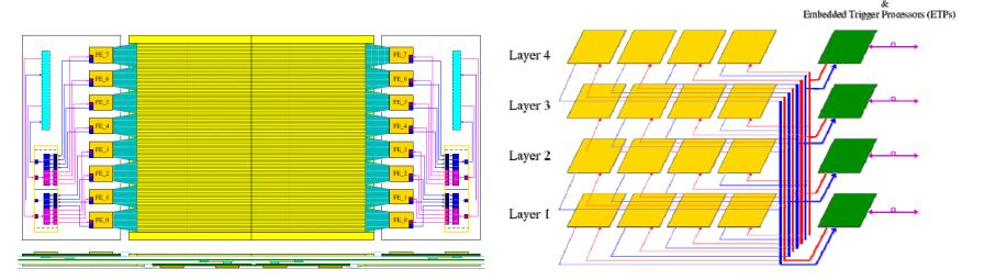
Phase II upgrade of the CMS Strip Tracker (trigger data readout and embedded trigger processors): data concentrators in the modules and high speed links between modules and trigger processors.
