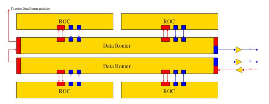
Phase II upgrade of the CMS pixel detector: two 640 Mbps electrical links from each ROC; two uplink optical fiber ( $\geq 1.6$  Gbps) for each 4-ROC module and one downlink optical fiber optionally shared among several modules.
