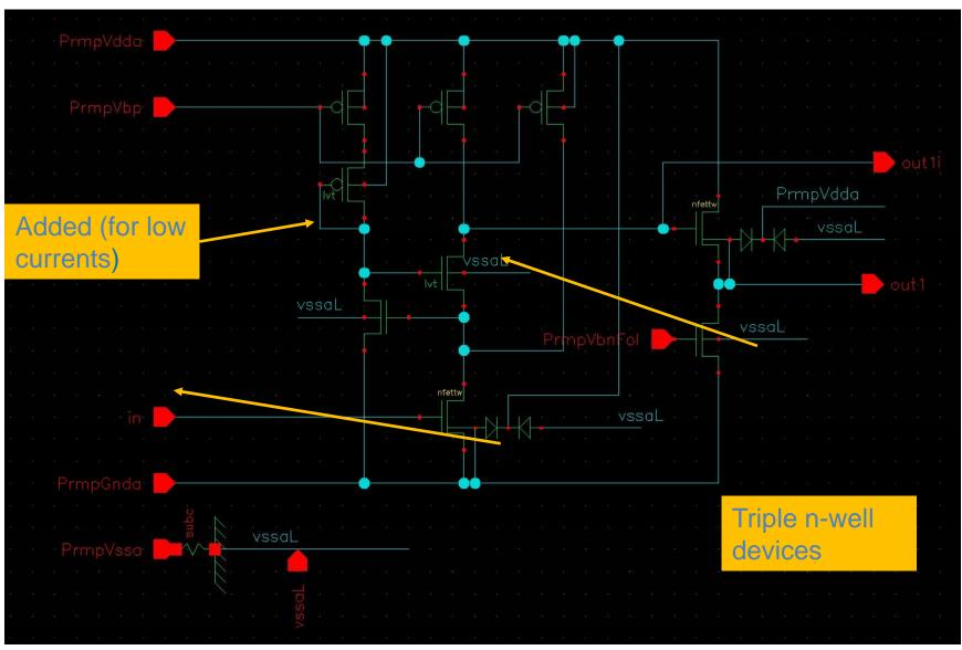
Straight regulated cascode, for electron collection (positive going output)
