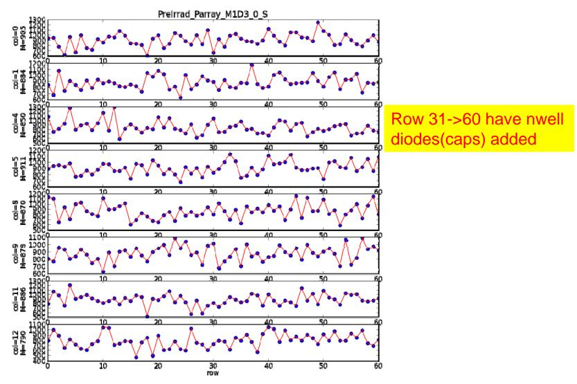
before irradiation measurements nominal setup @ 17µa/cell
