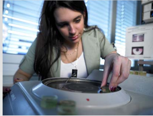
Polishing of Micro Section
