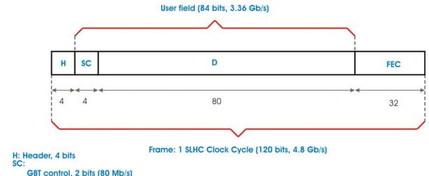
GBT control, 2 bits (80 Mb/s) Slow control port, 2bits (80 Mb/s) D: DATA/TTC/EC - User data, 80 bits (3.2 Gb/s) FEC: Forward Error correction, 32 bits
