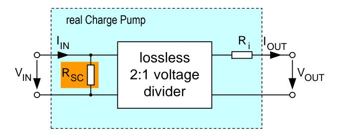
Ideal 2:1 converter ( $V_{out}=V_{in}/2$ ,  $I_{out}=2*I_{in}$ ) with shunt resistor and output resistor
