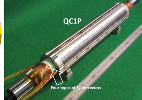
IR with \beta_y^* = 0.3mm SC final focus system
