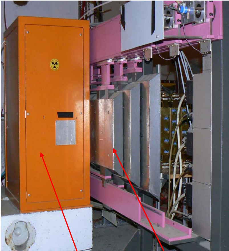
The Cs 137 source container The external screens and collimators
