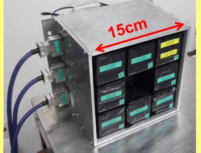
■Volume:10cm × 10cm × 15cm ■Gas:Ar 90% +  $C_2H_6$  10% 1atm (sealed) ■ Position resolution: 200µm ■ Energy resolution: 28% (FWHM) @ 31keV Stable gas gain:  $\sim$ 36000(µ–PIC  $\sim$ 3600 GEM  $\sim$ 10)
