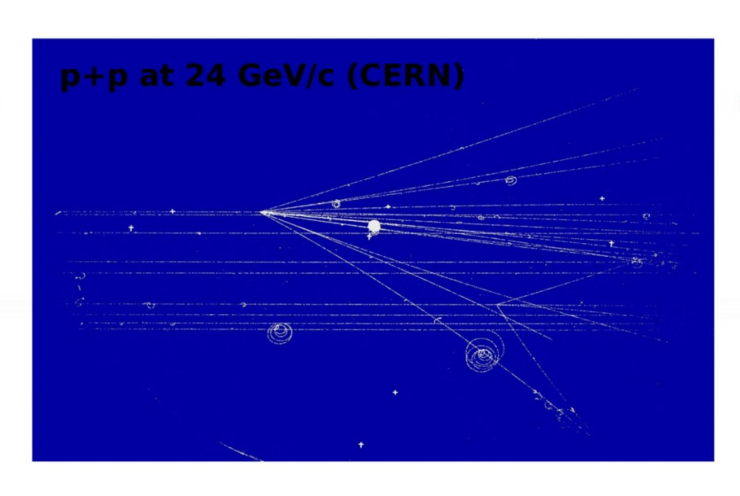
LIQUIDE HYDROGEN SERVES AS TARGET AND DETECTOR
