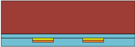
1. Wafer with buried TSV landing pads
