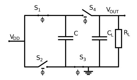
Introduction to step-up charge pump circuits
