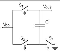
$$(V_{OUT} - V_{DD}) C = V_{DD} C$$
