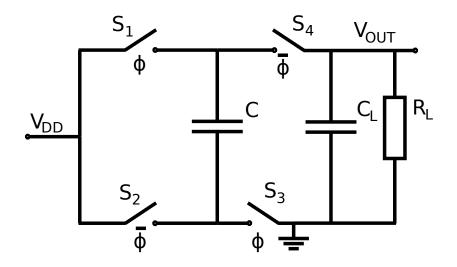
Introduction to step-up charge pump circuits
