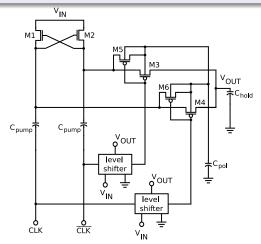
An integrated DC-DC step-up charge pump for the serial powering scheme in ABCN (130nm) Voltage doubler for serial powering scheme
