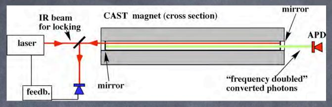
Cavity mirrors placed in chambers at opposite sides of the magnet to form a cavity
