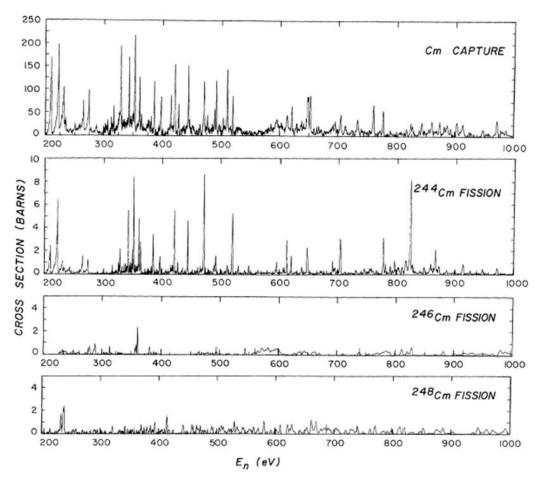
This experiment was performed with the neutron time-of-flight (TOF) method in 1969 **using a under-ground nuclear explosion (one single pulse)** as a pulsed neutron source and Moxon-Rae detectors operated in current mode.
