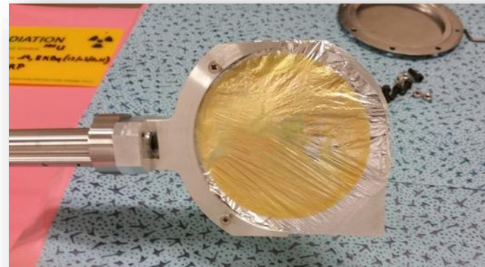
Target: thin layer of ^{235}\text{U} deposited on an Al support of 0.75\ \mu\text{m} thickness
