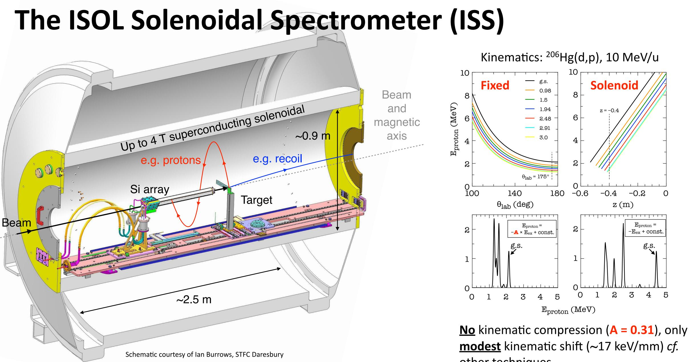
For this measurement the Si array used in the comparable HELIOS spectrometer at Argonne National Laboratory will be used in place of the one shown in this schematic.
