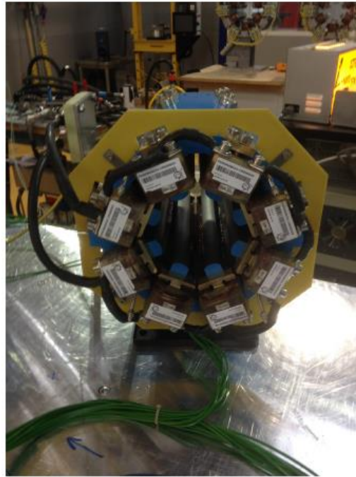
OCTFF2 mounted on Magnetic Measurements bench
