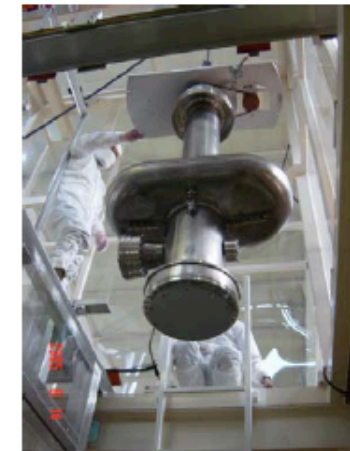
High Pressure Water Rinsing
