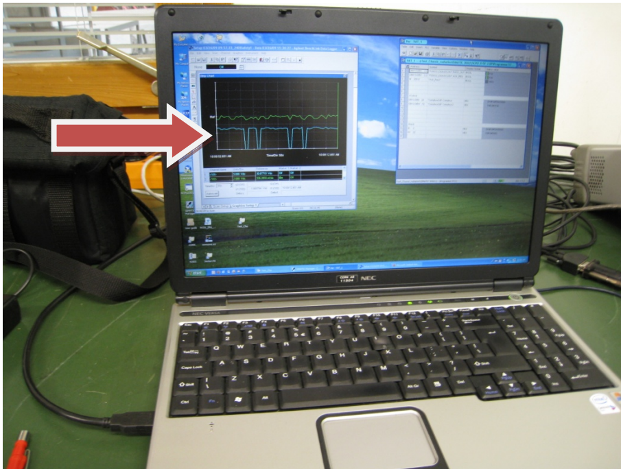
Figure 4 : Four Single Event Functional Interrupts of the SIEMENS 24 DI remote input module SM326 clearly visible via the on line readout system.
