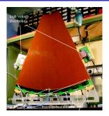
Large GEM chamber ( $66 \times 66$  cm) based on two novel techniques: single mask technique and GEM splicing.
