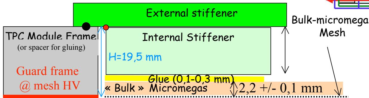
**Module assembly :** bulk-micromegas gluing on mechanical stiffener with control of the H=19,5 mm dimension, HV filter integration, mechanical metrology and gas tightness Q/C (1 module / day)
