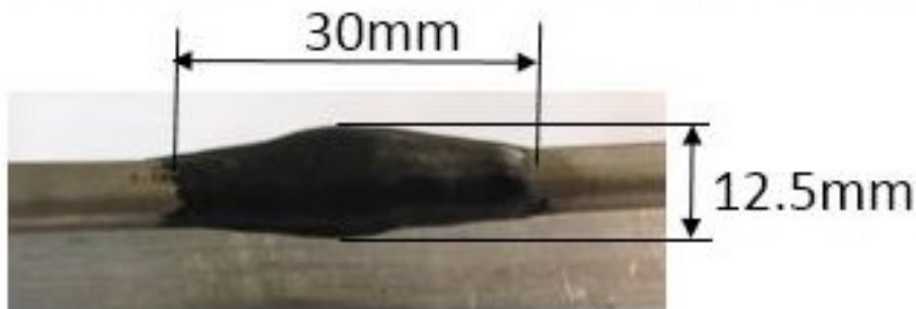
Epoxy over the joint
