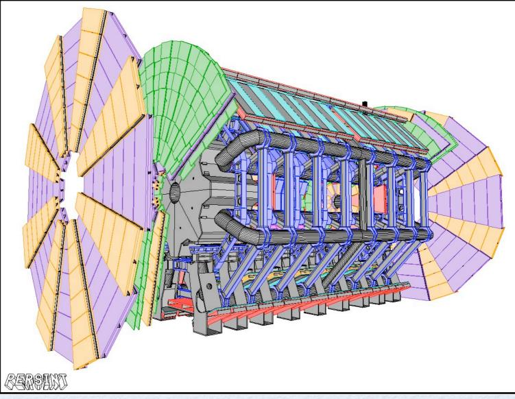
Magnet System -Barrel and 2 Endcap Toroids
