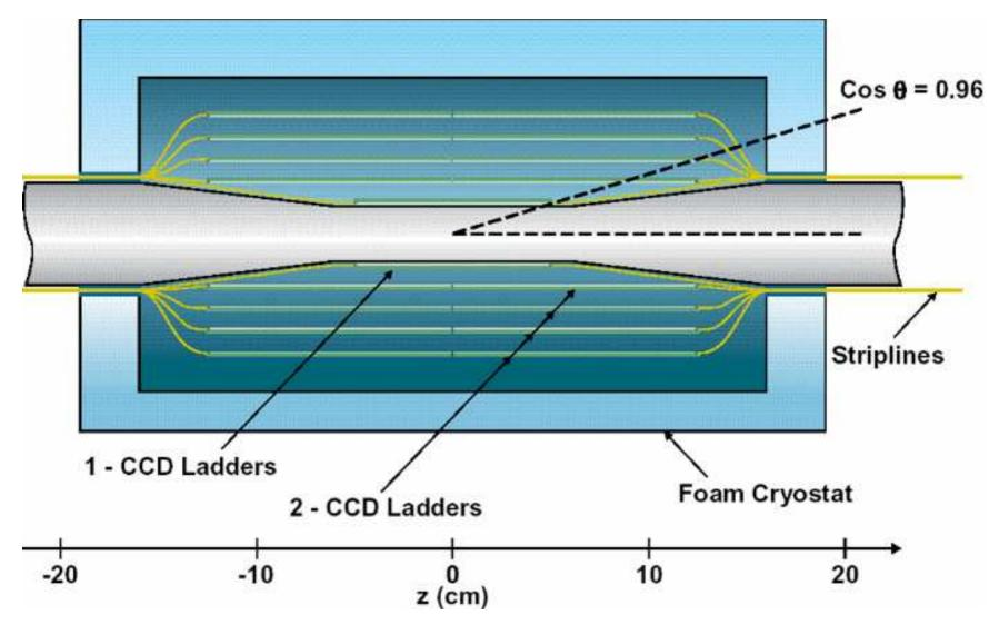
CCD layers at 15, 26, 37, 48 and 60 mm. Each layer  $< 0.1\% X_0$ .
