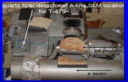
Prototype quartz fiber detector (8 x 100  $\mu$ m, 8 x 600  $\mu$ m, with multi-anode PMT is installed in the A-line SLM
