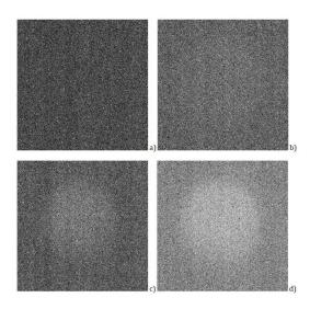
Surprising radiation from Pirani vacuum gauges was observed at ring region on CCD.
