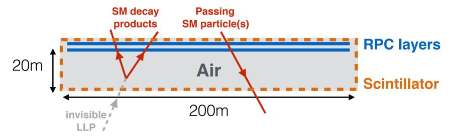
Layers of RPCs in the roof act as a directional **tracker**. Scintillators give additional **veto**. ~ns timing, ~cm position resolution.
