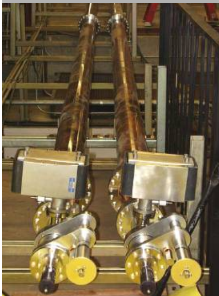
The ASTA pulse compressor with variable iris
