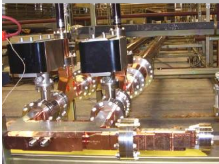
The ASTA pulse compressor with variable iris
