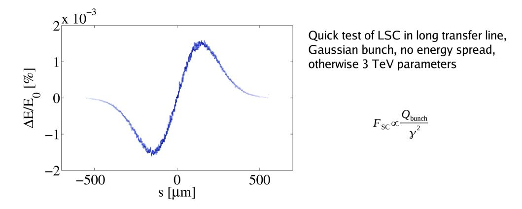
Space charge forces might influence transverse and longitudinal momentum. Due to the large beam energy of 8-9 GeV they should be small but a detailed study remains to be done using a more realistic bunch profile.
