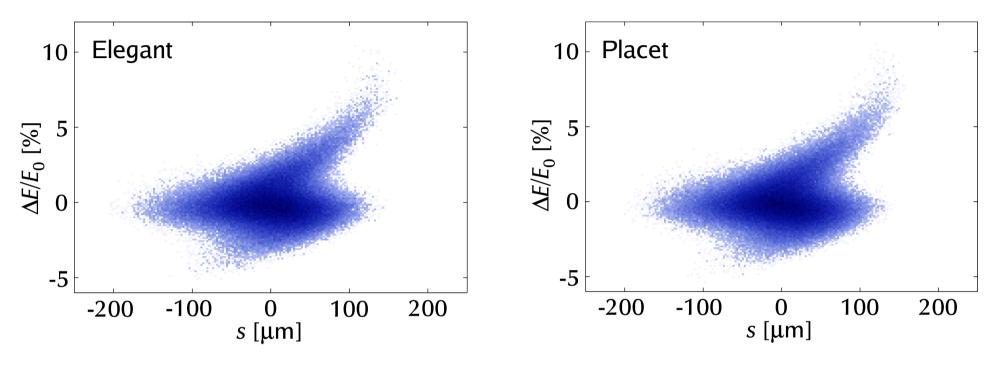
ISR, wake fields and chromatic effects lead to an emittance growth in the horizontal plane of  $\Delta \varepsilon_{nx} = 50 \text{ nm rad}$  (Elegant) and  $\Delta \varepsilon_{nx} = 60 \text{ nm rad}$  (Placet). Emittance in vertical plane is unchanged.
