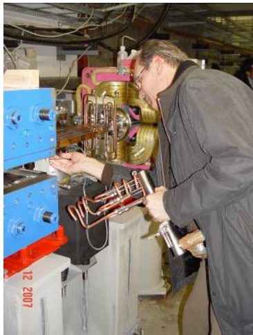
Regular absorbers of 26kW for PETRA-III project
