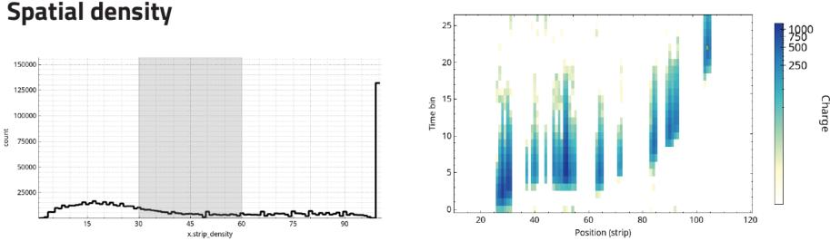
Spatial density is defined as percentage of valid strips out of the total strip span. Such events are either very noisy or likely indicate a high energy conversion electron.
